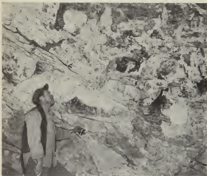
FIG. 22. Graphic granite underlain by very coarse-grained perthite-quartz pegmatite, El Molino mine. Separating these two units is 18 inches of finer-grained pegmatite composed of abundant masses of graphic granite in a matrix of quartz, albite, and muscovite.
